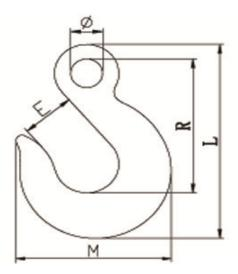
ر1:18mm R±2:86.5mm L±3:124mm M±2:89.5mm E±2:33mm
